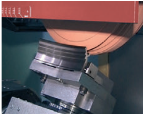
Shroud segment – multiple operations in 1 set-up
