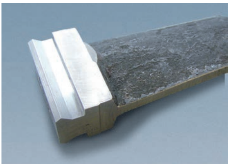
Compressor blade – multiple operations in one set-up
