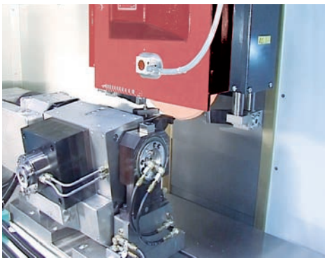
Compressor blade – multiple operations in one set-up
