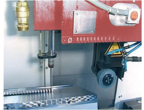
Measuring probe, pneumatically retracting from measuring position, up to 2 ½ axes, measuring accuracy +/- 1 µm
