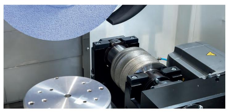
The large table dressing device enables the mounting of wide diamond rolls The two bearings and the servo motor drive enable reliable dressing across with a multitude of machining profiles for different workpieces and makes a the entire speed range. significant contribution to minimizing changeover times.
