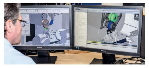
A SIEMENS NX postprocessor is available for CAM process development. The generated NC programs take account of the MÄGERLE grinding cycles. As a result the programs can be easily edited on the machine control unit via operator guidance. MÄGERLE provides a Vericut package for simulating and checking the programs.
