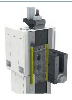
The unique design principle of MÄGERLE machining centers forms the basis for the overall machine quality. The vertical axis is supported by hydrostatic wrap-around guideways on a thin oil film and is completely separated from the column's upper section. This principle enables the machines to withstand very high stresses free of wear, even in long-term use. The oil film also has a vibration-damping effect and guarantees highprecision machining of simple or complex workpieces.
