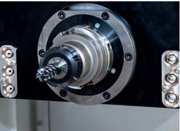
The NC controls of the MÄGERLE grinding centers enable precise positioning of the coolant supply, taking into account the respective grinding wheel geometry. Nozzles are available on the grinding support for milling/drilling tools, and a coolant supply can be optionally provided through the
