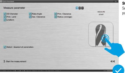
Select/deselect required measurement parameters and start measurement
